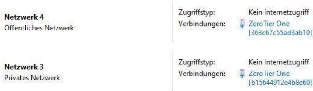
Fig. 12: Screenshot of two ZeroTier adapter in network control center in MS Windows
